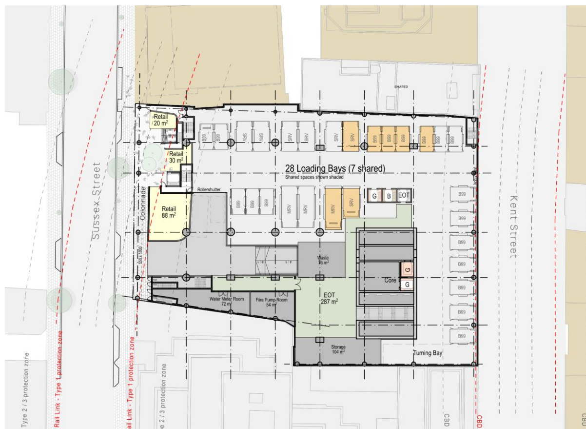
Figure 24: Indicative Shared Loading Arrangement
